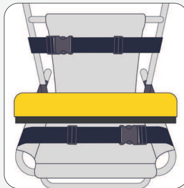
2. Ensure the chair safety straps are fastened and placed onto the zipped hammock. Place Comfy Seat onto the frame and secure.
